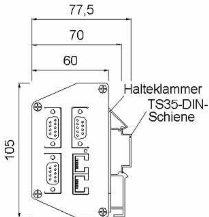
EASY2505 in aluminium housing – front and side view
